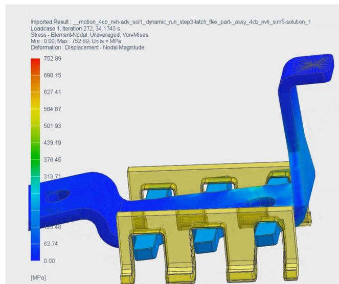
Motion model of a latch using a flexible body.
