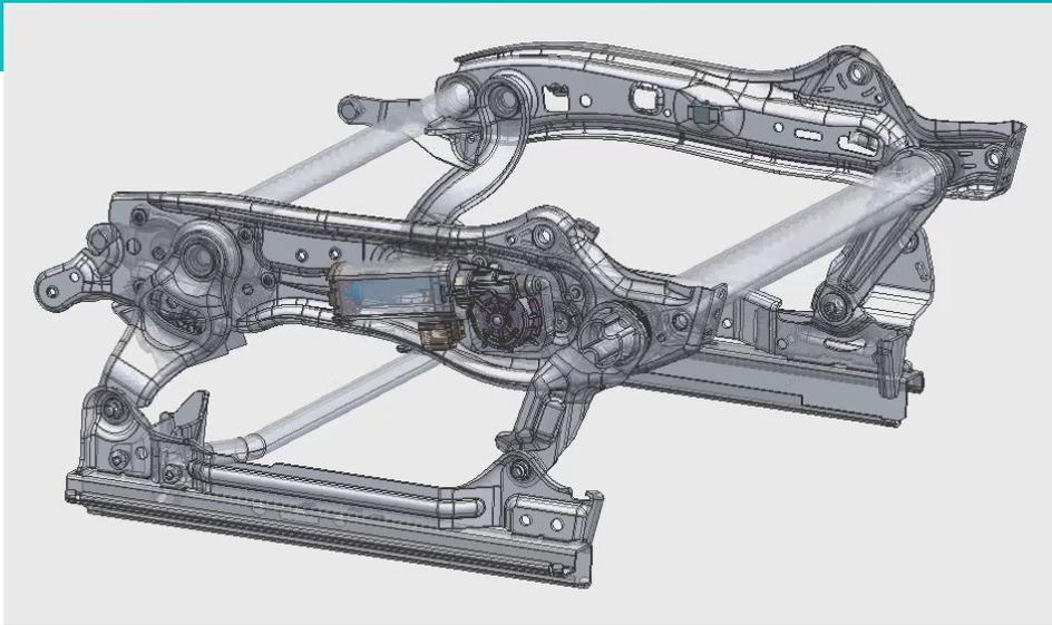
Seat geometry with e-Pump mechanism attached.
