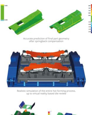
PAM-STAMP enables detailed analysis of the influence of tool deformation on the final springback
