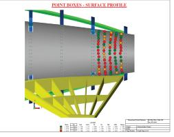
Point Boxes - Surface Profile Use color coding for quick analysis and communication of surface profile variation and pass/fail conditions.
