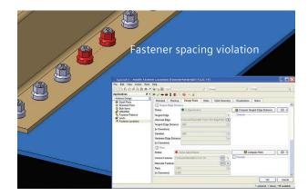
Syncrofit automatically detects and calculates the spacing between fasteners to ensure pitch requirements have been satisfied.
